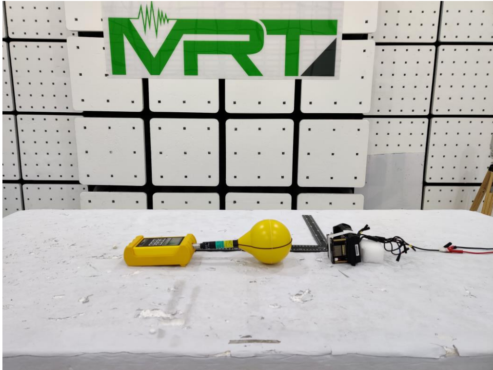
Description: RF Exposure Test Setup for Magnetic Field Emissions WPT Test Mode 3
