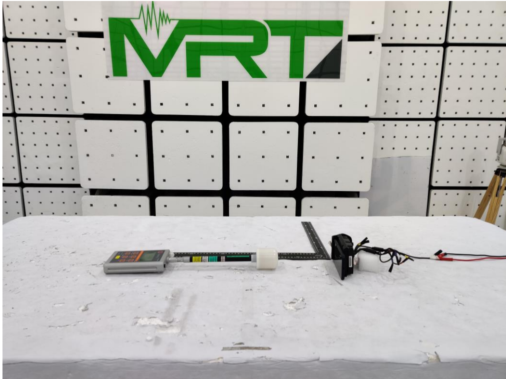
Description: RF Exposure Test Setup for Magnetic Field Emissions WPT Test Mode 1
