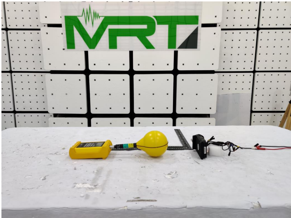
Description: RF Exposure Test Setup for Magnetic Field Emissions WPT Test Mode 1
