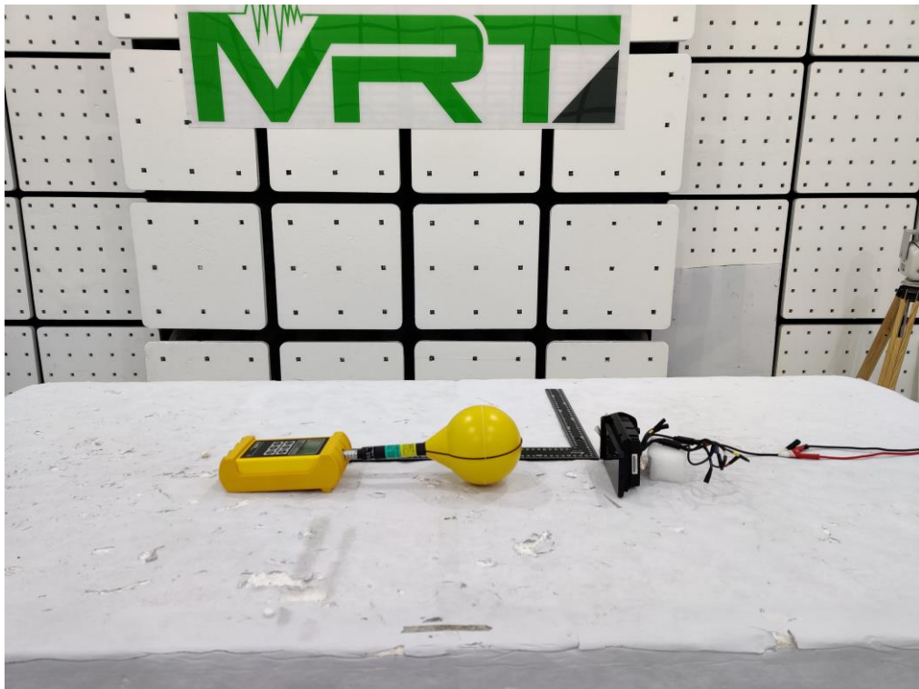
Description: RF Exposure Test Setup for Magnetic Field Emissions WPT Test Mode 3
