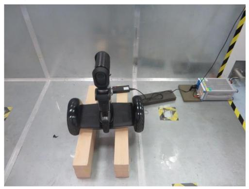
Description: Conducted Emission Test Setup
