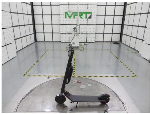
Description: Radiated Spurious Emission Test Setup for  $30MHz \sim 1GHz$
