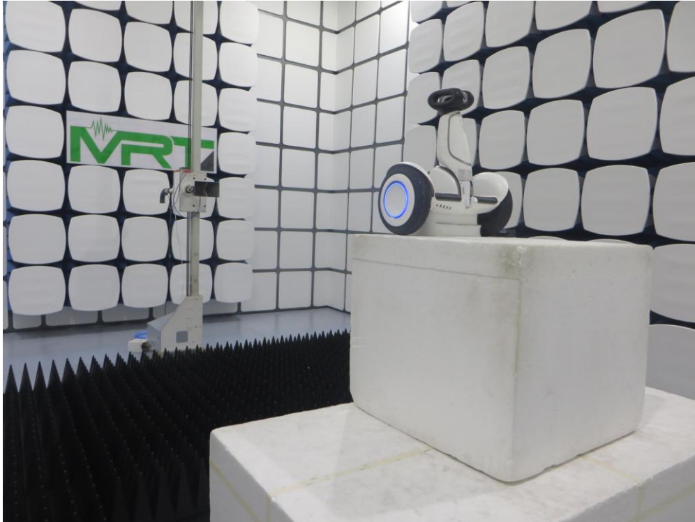
Description: Radiated Emission Test Setup for 18GHz ~ 40GHz (Bluetooth Testing)
