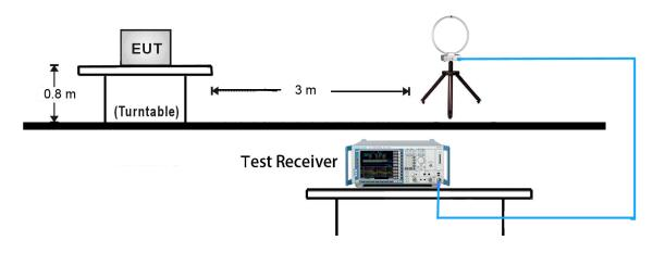
30MHz ~ 1GHz Test Setup:
