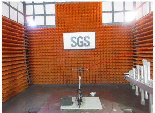
RF antenna and module are located in the handle at above 0.8m from the floor.
