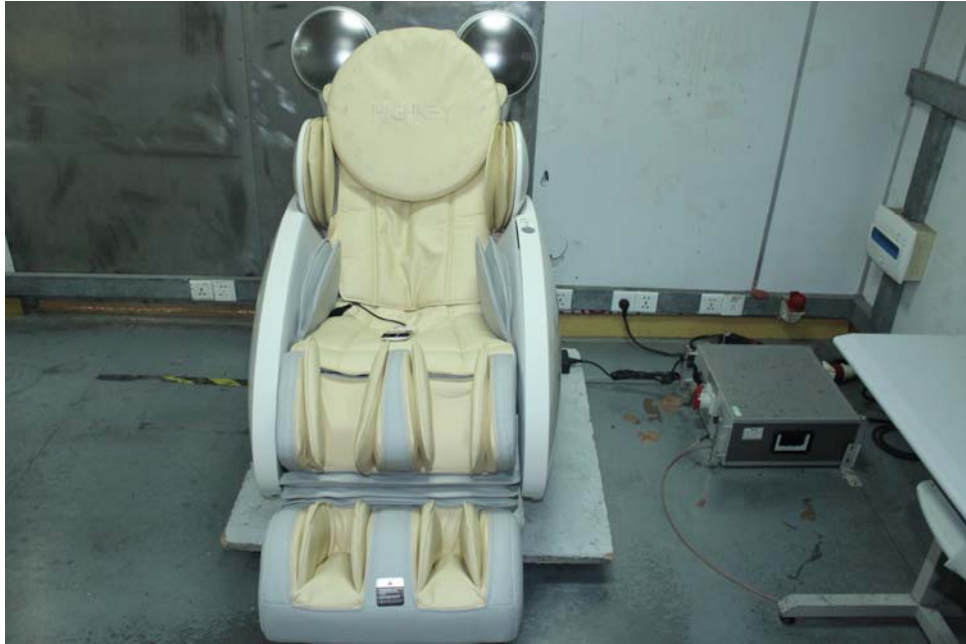
Photograph of set-up for conducted Emission
