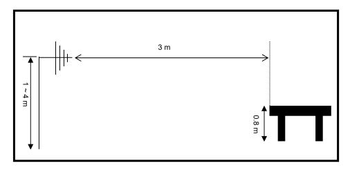
Radiated emission setup, above 1 GHz
