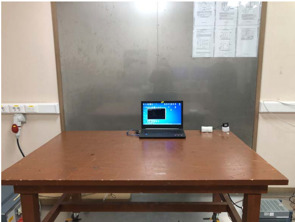
Conducted emission measurement (Front)
