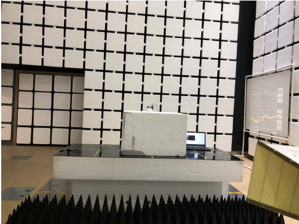
Radiated RF measurement (Above 1 GHz)
