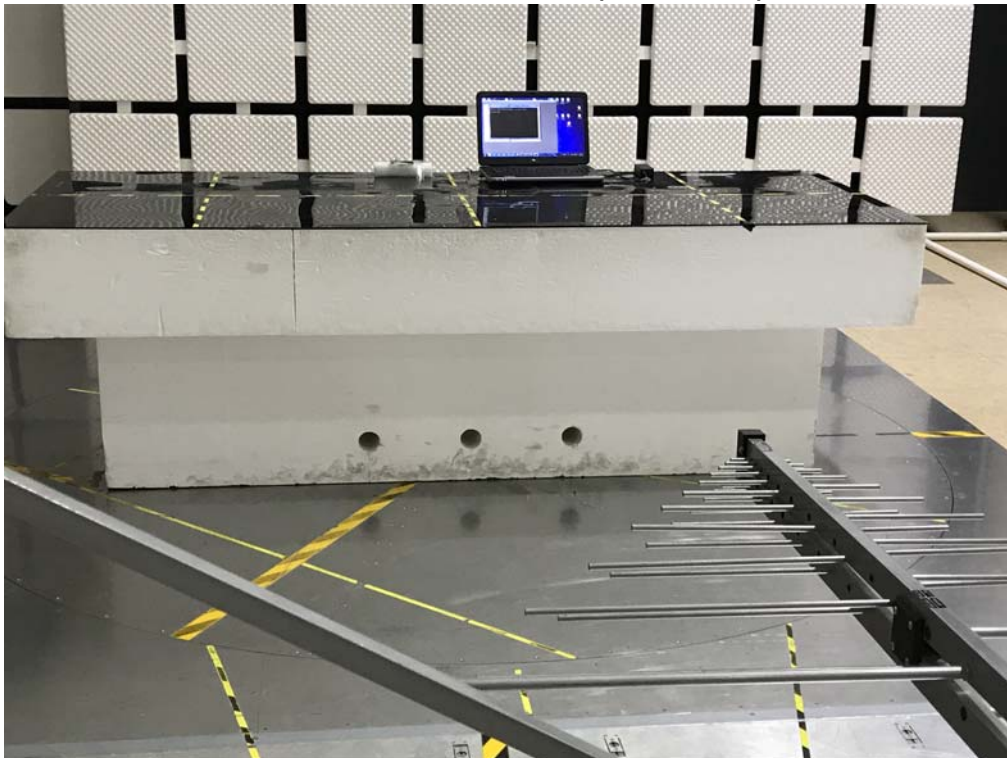
Radiated RF measurement (30 MHz - 1 GHz)
