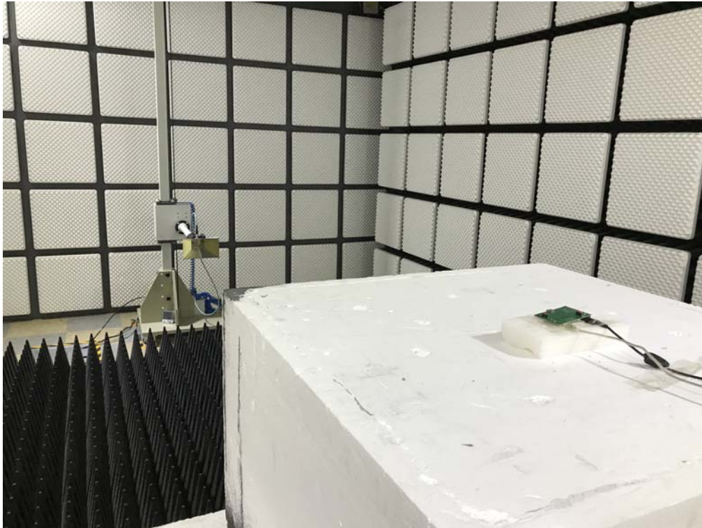
Radiated RF measurement (Above 1 GHz)
