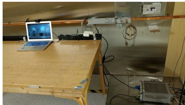
Test setup for conducted Emission test: Measured with AC/DC adapter Model A1435 and Mac Model A1466, S/N C02PG6ZPG941
