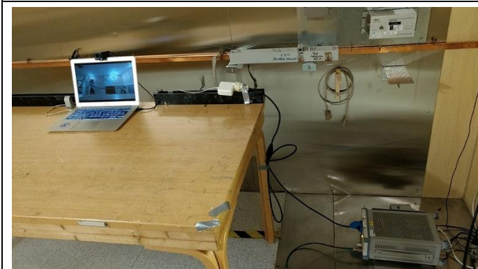
Test setup for conducted Emission test: Measured with AC/DC adapter Model A1435 and Mac Model A1466, S/N C02PG6ZPG941
