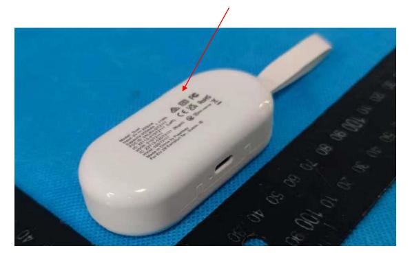
Because the Bluetooth Earphones is too small, the FCC ID number can only be printed on the charging box.
