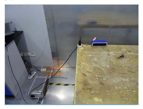
Photograph – Radiation Spurious Emission Test Setup
