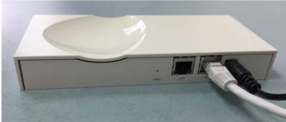
Figure 6: Power and ETH2 connections
