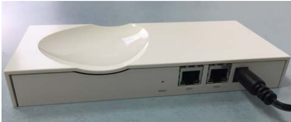
Figure 4: Router mode power connection
