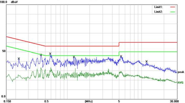
Note: The charging of < 1% Battery, 50% Battery, >99% Battery all has been tested, the worst case is charging of < 1% Battery, only shown the worst case in this report.
