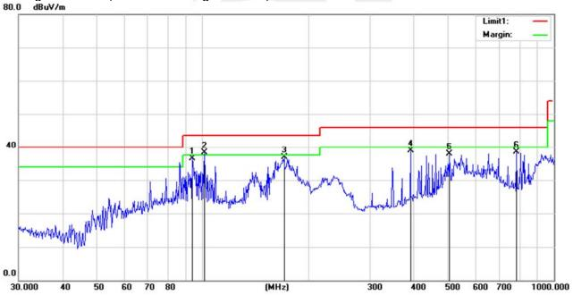
Note: The charging of < 1% Battery, 50% Battery, >99% Battery all has been tested, the worst case is charging of < 1% Battery, only shown the worst case in this report.
