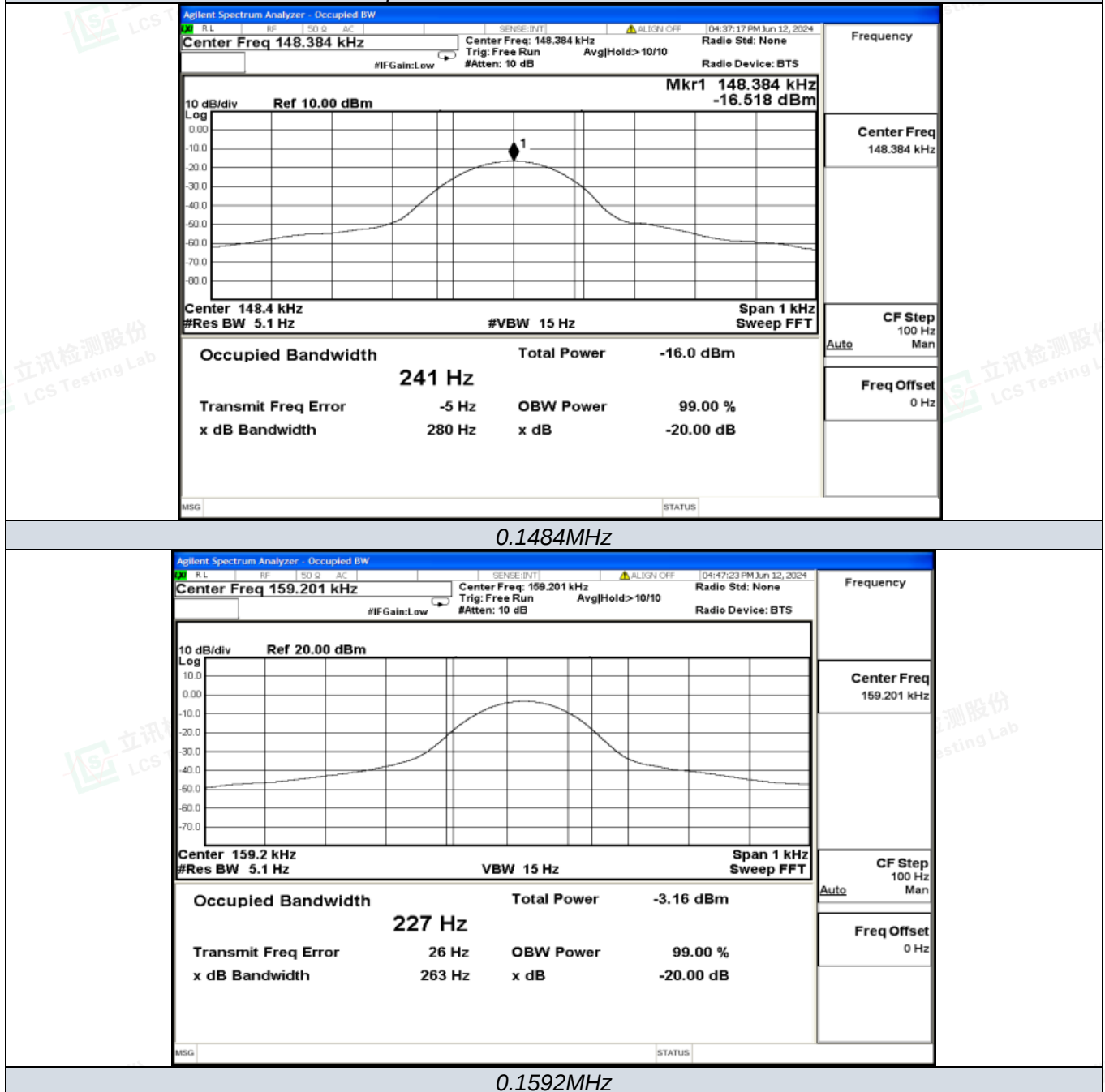
Test plot of 20 dB Bandwidth Measurement
