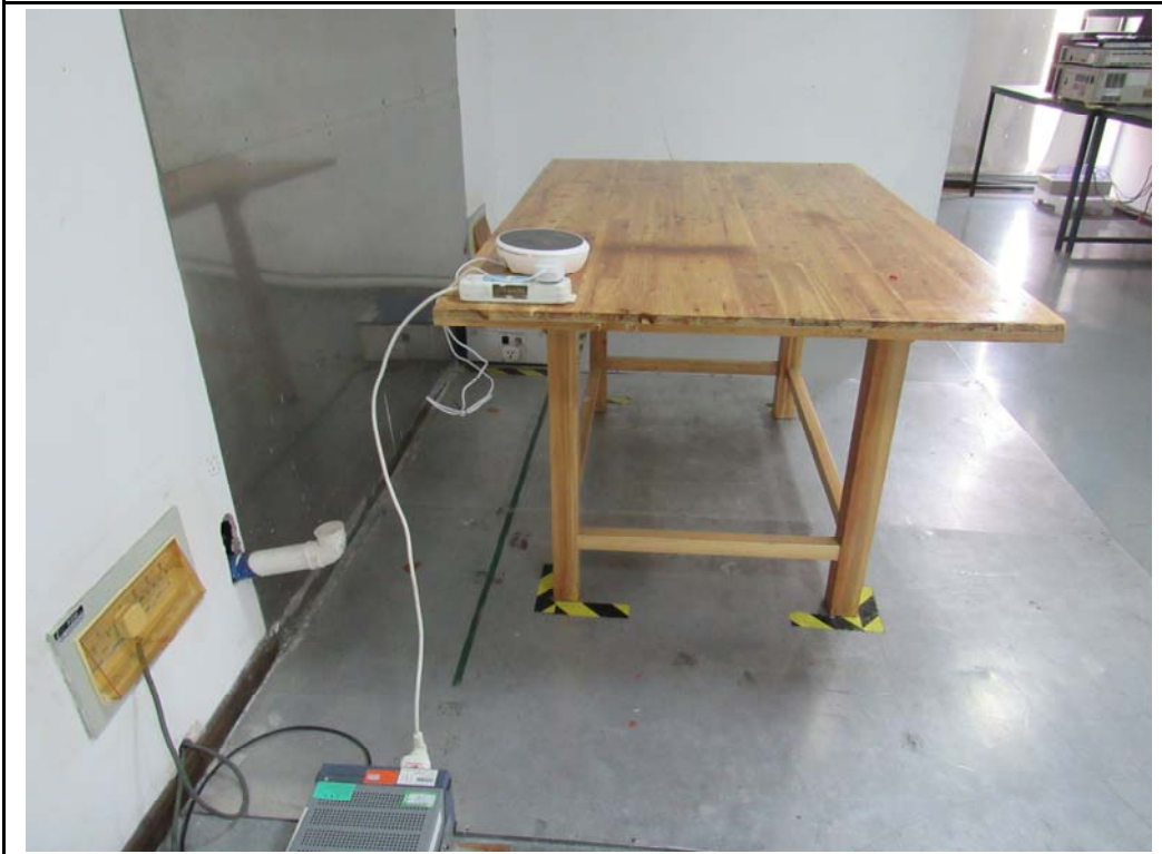
Conducted Emissions Test Setup Side View
