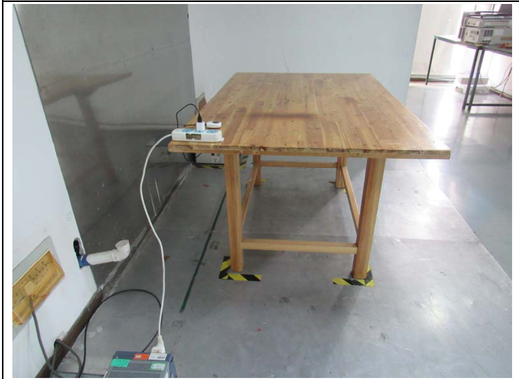
Conducted Emissions Test Setup Side View
