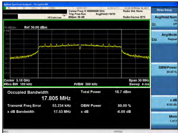
(802.11ac20) -6dB Bandwidth plot on channel 40
