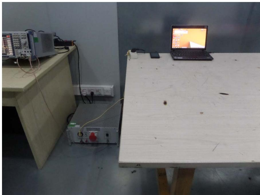
**Radiation Emission Test Setup (30MHz to 1GHz)**
