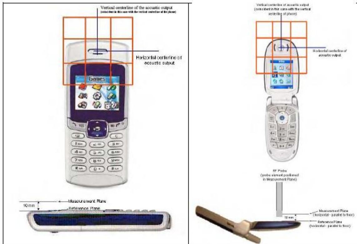
Reference and plane for RF emission measurements
