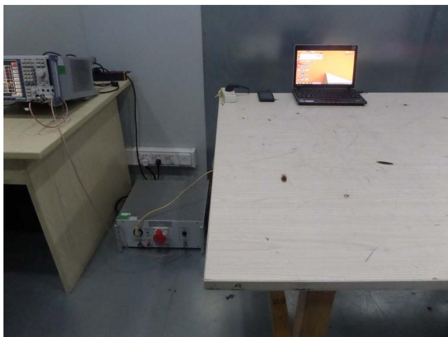
**Radiation Emission Test Setup (30MHz to 1GHz)**
