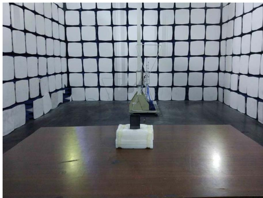
**Radiation Emission Test Setup (Above 1GHz)**
