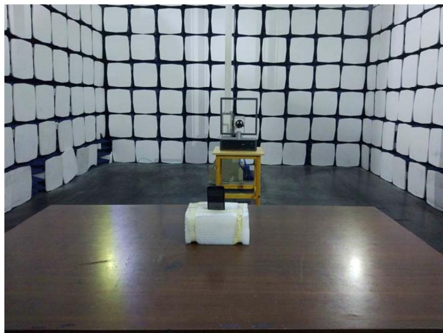
**Radiation Emission Test Setup (30MHz to 1GHz)**
