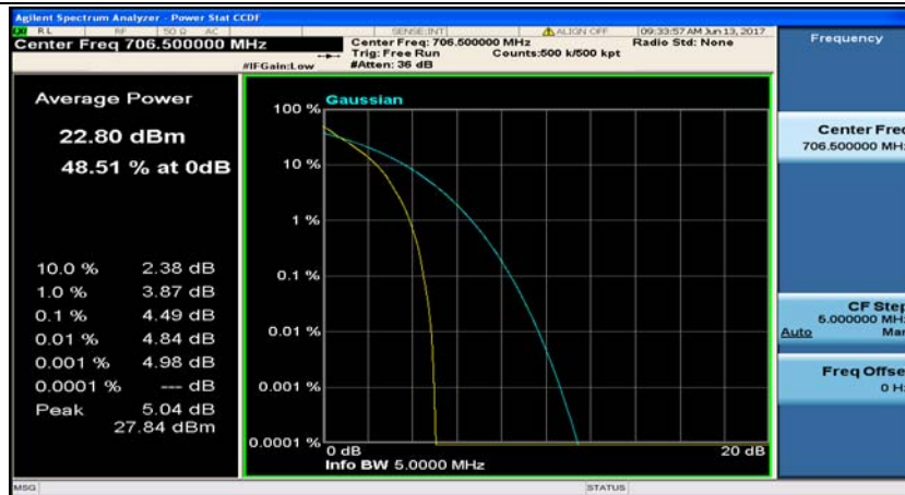
(Channel Bandwidth: 5 MHz)_LCH_QPSK_12RB#6
