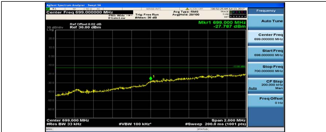
(Channel Bandwidth: 3 MHz)_LCH_QPSK_15RB#0
