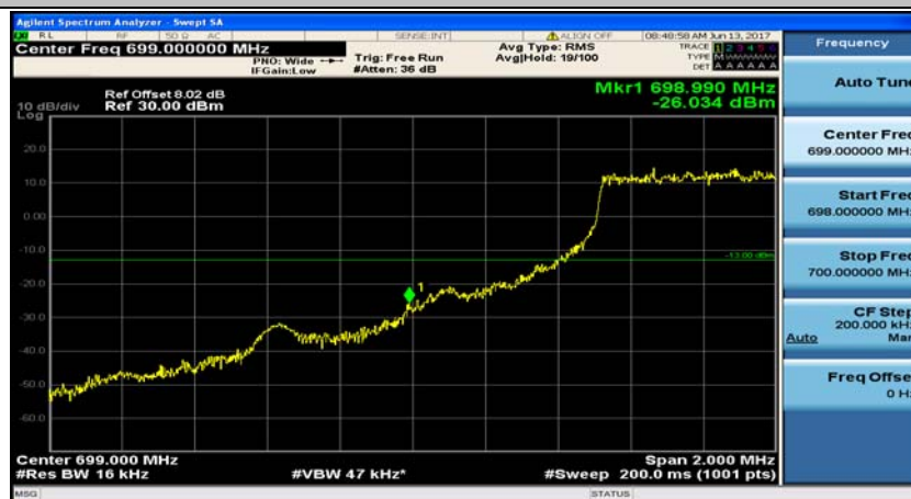
(Channel Bandwidth: 1.4 MHz)_LCH_QPSK_3RB#3
