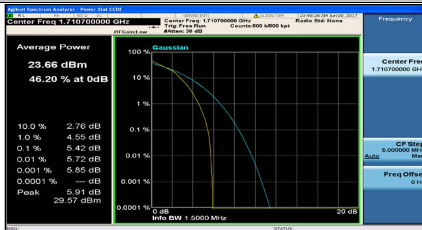
(Channel Bandwidth: 1.4 MHz)_LCH_16QAM_6RB#0
