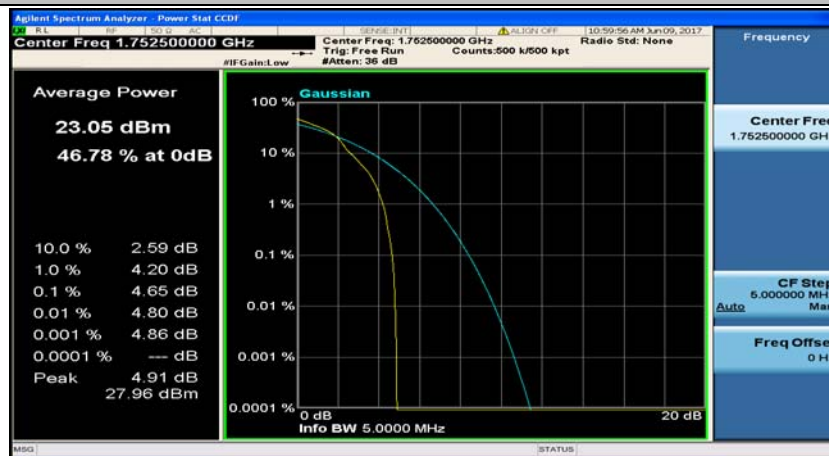
(Channel Bandwidth: 5 MHz)_HCH_16QAM_12RB#0
