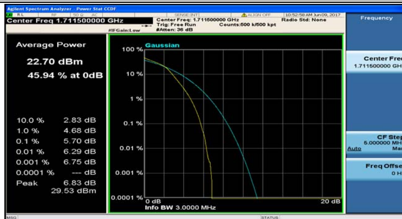
(Channel Bandwidth: 3 MHz)_LCH_16QAM_15RB#0
