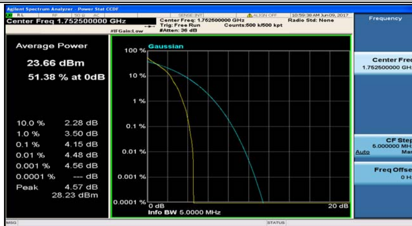
(Channel Bandwidth: 5 MHz)_HCH_QPSK_12RB#0
