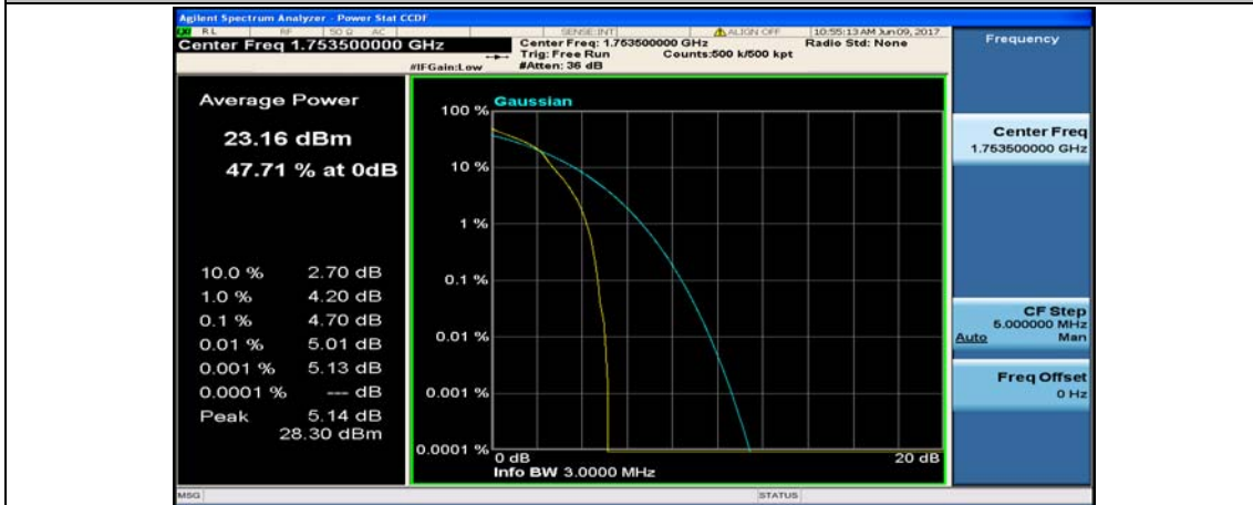
(Channel Bandwidth: 3 MHz)_HCH_16QAM_1RB#7
