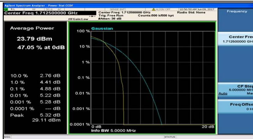
(Channel Bandwidth: 5 MHz)_LCH_16QAM_1RB#24
