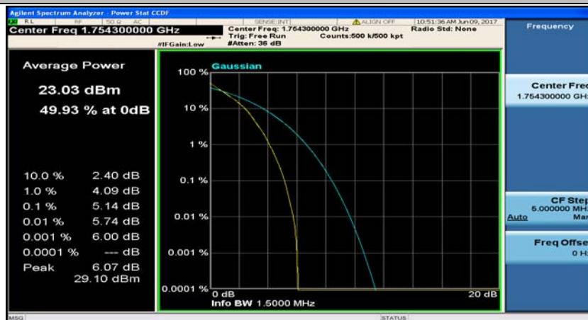
(Channel Bandwidth: 1.4 MHz)_LCH_16QAM_1RB#0
