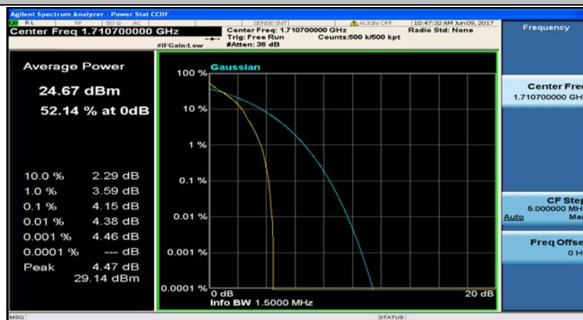
(Channel Bandwidth: 1.4 MHz)_LCH_QPSK_3RB#0
