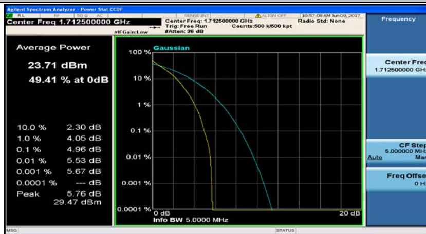
(Channel Bandwidth: 5 MHz)_LCH_QPSK_12RB#13
