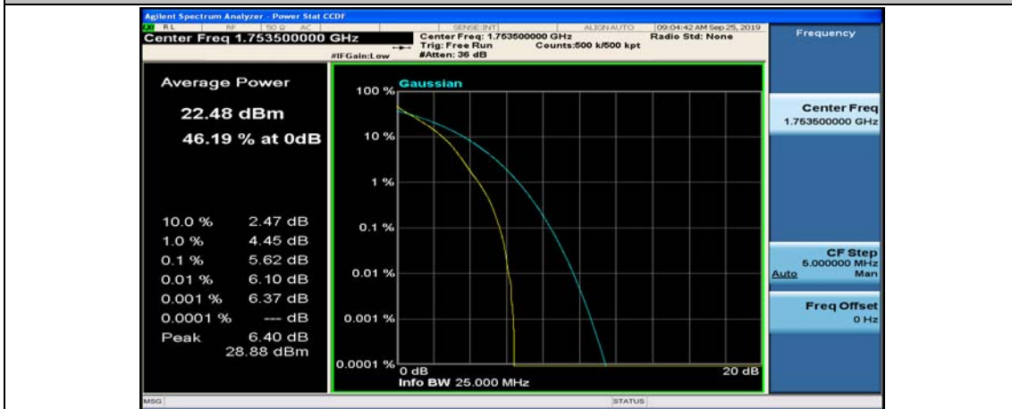
(Channel Bandwidth: 3 MHz)_HCH_QPSK_15RB#0
