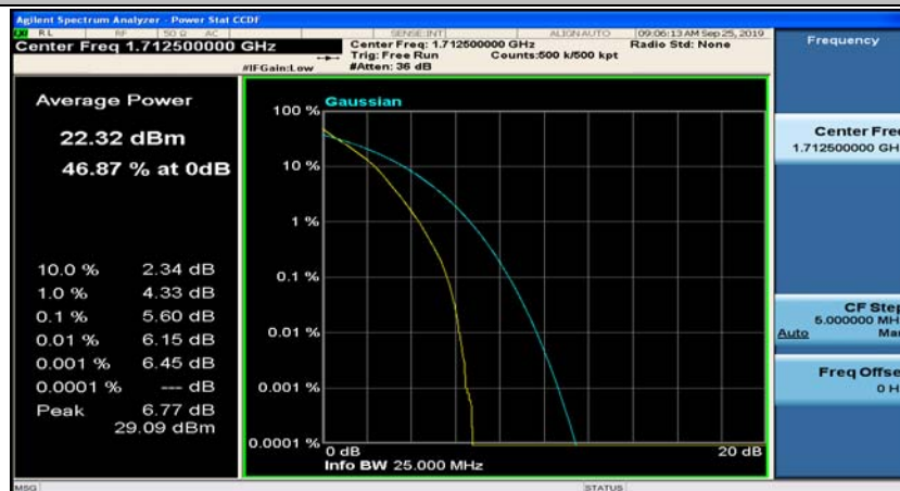
(Channel Bandwidth: 5 MHz)_LCH_QPSK_25RB#0
