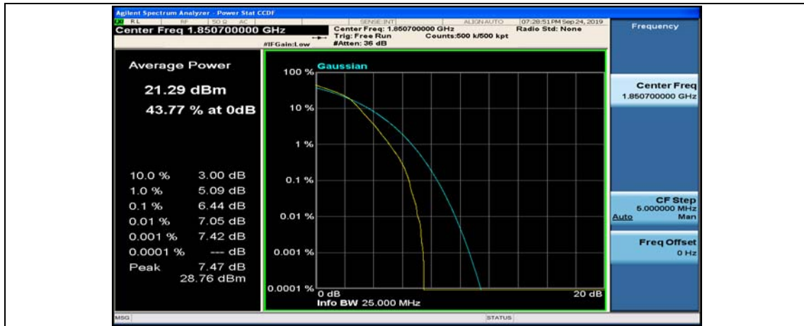
(Channel Bandwidth: 1.4 MHz)_MCH_16QAM_1RB#0
