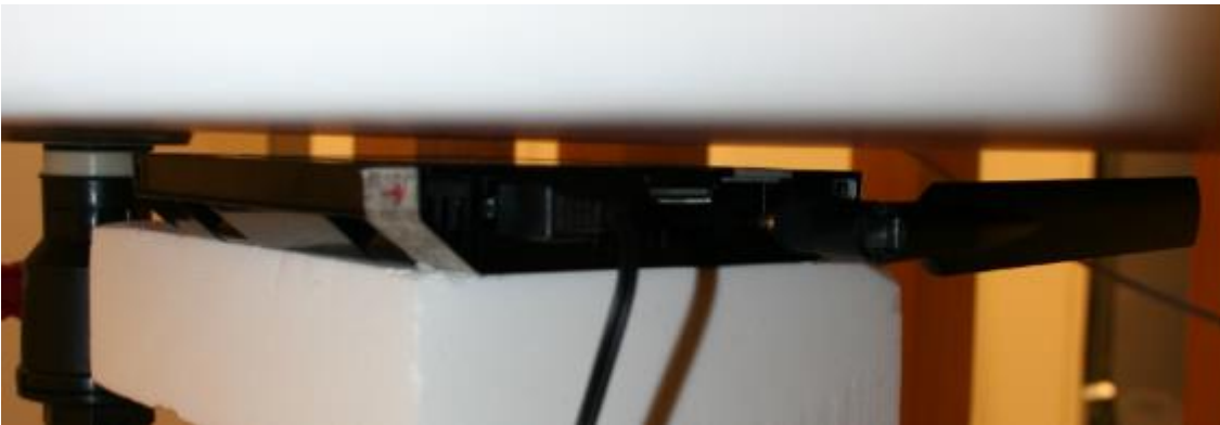
Figure 9. Test position used for testing; device under test with antenna tilted horizontally to rightside.
