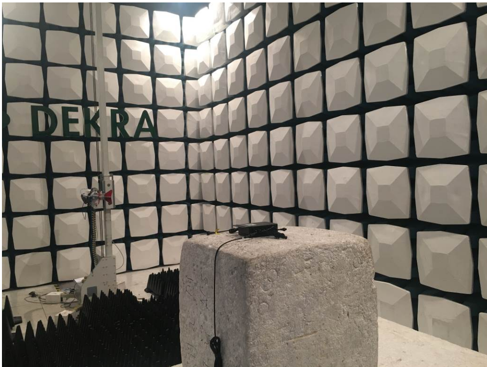
Description: Radiated Emission Test Setup for 1~18GHz
