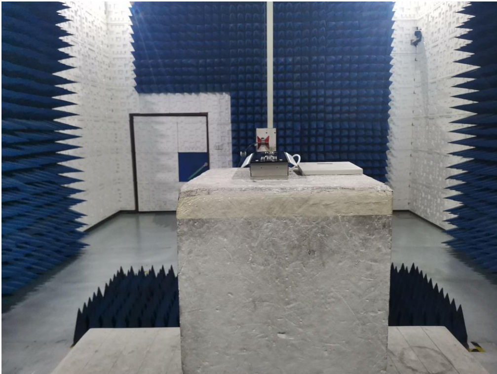
FCC RADIATED EMISSION TEST SETUP ABOVE 1GHZ
