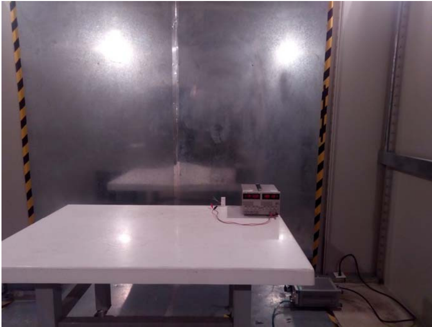
Conducted Emissions - Front View
