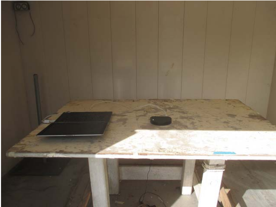
Figure 1 EUT Configuration for Radiated Emission Test
