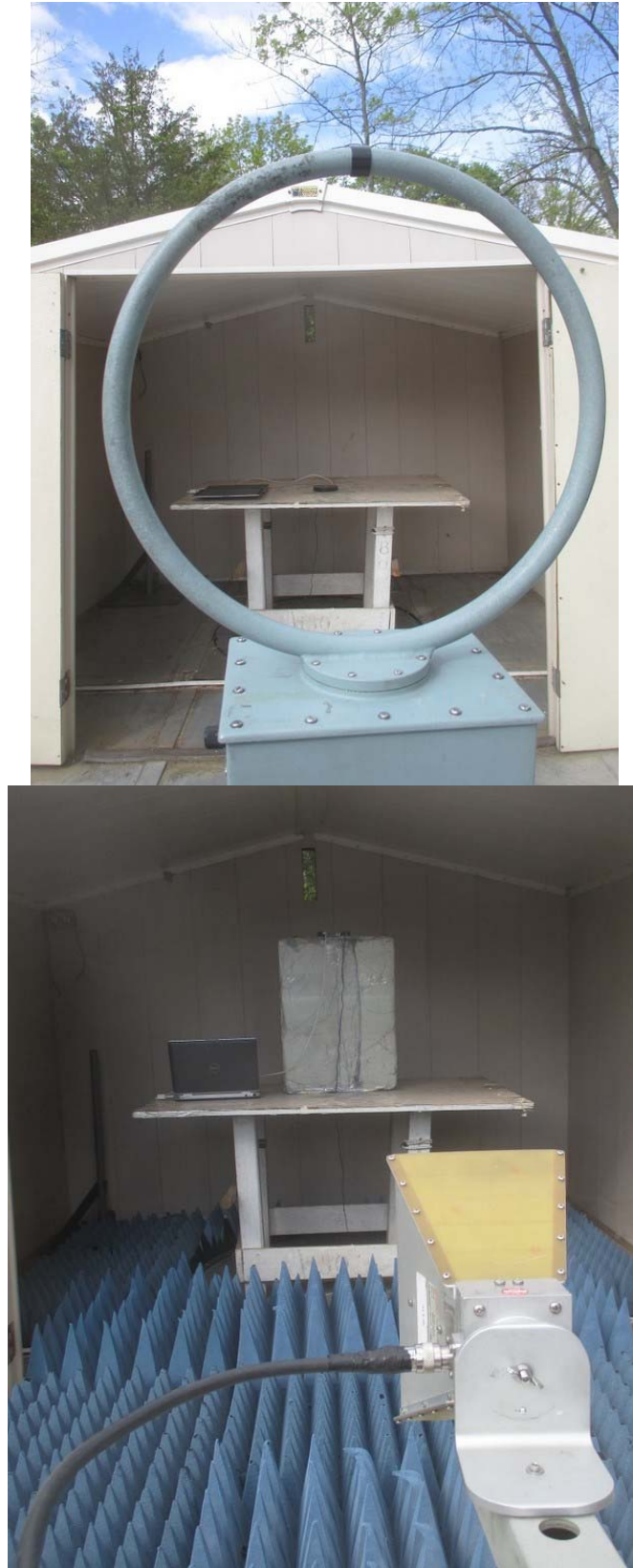
Figure 2 Radiated Emission Test Setup
