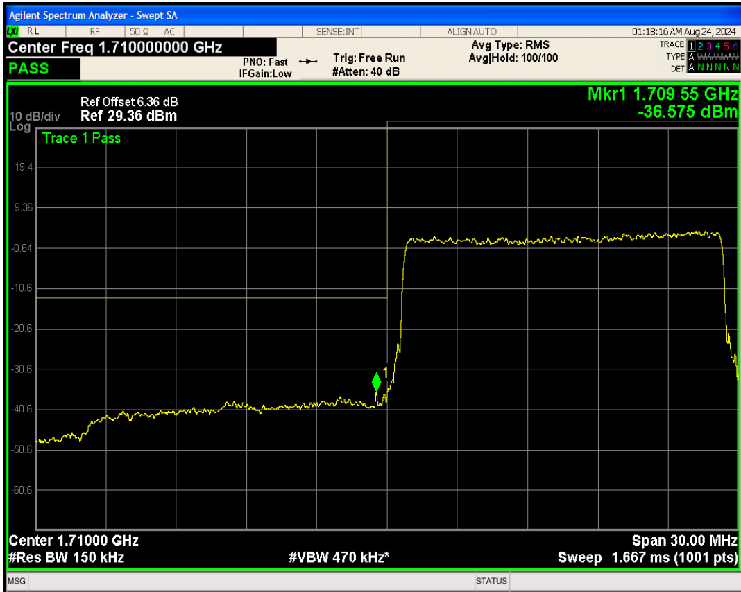
Band66 16QAM BW=15MHz Channel=132047 RB Size=75 Position=#0
