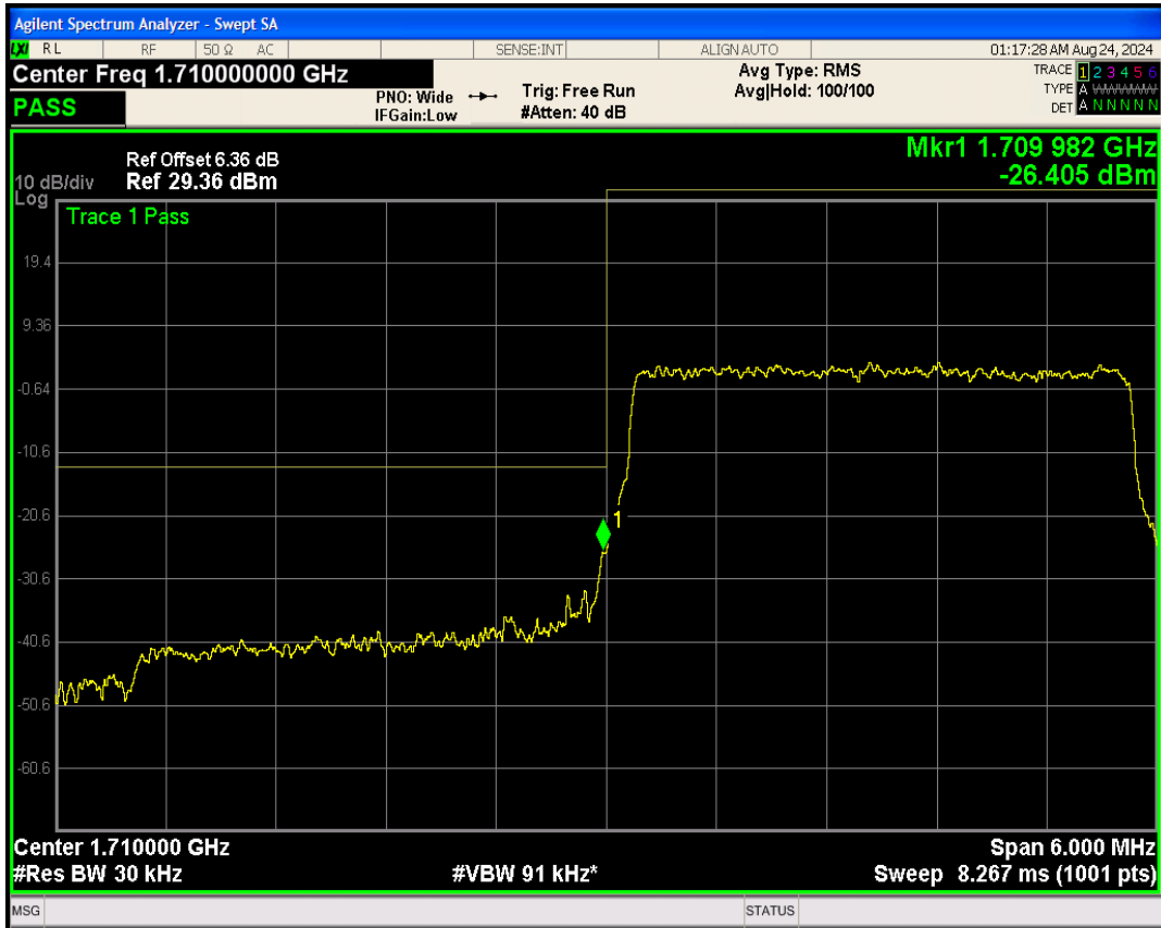
Band66 16QAM BW=3MHz Channel=131987 RB Size=15 Position=#0
