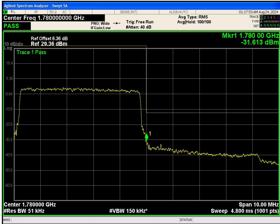
Band66 16QAM BW=5MHz Channel=132647 RB Size=25 Position=#0
