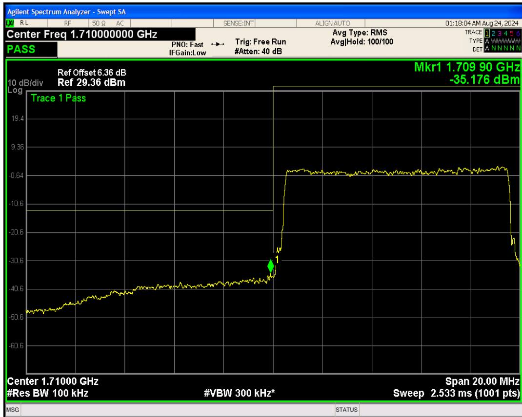
Band66 QPSK BW=10MHz Channel=132622 RB Size=50 Position=#0
