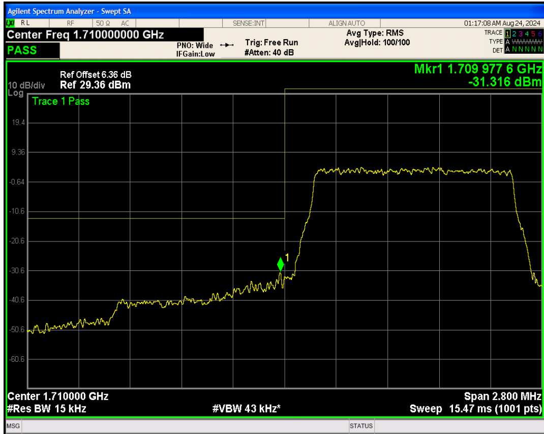
Band66 16QAM BW=1.4MHz Channel=131979 RB Size=6 Position=#0
