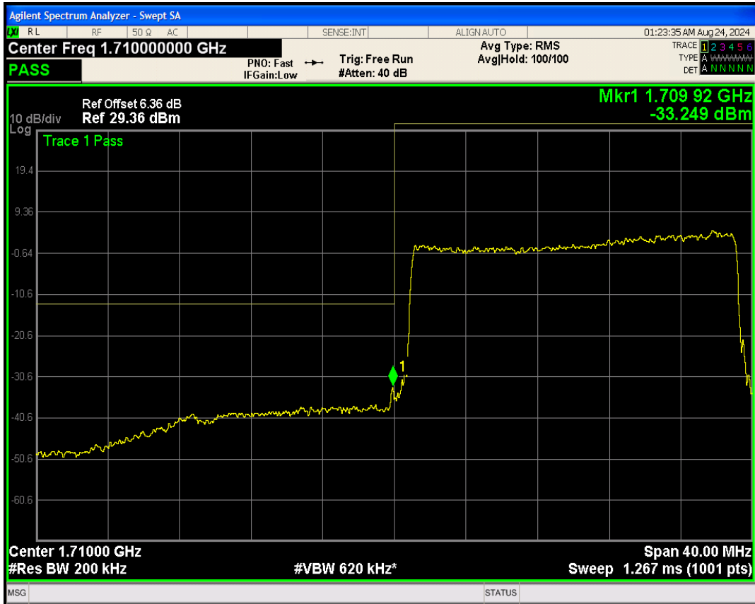
Band66 16QAM BW=20MHz Channel=132072 RB Size=100 Position=#0
