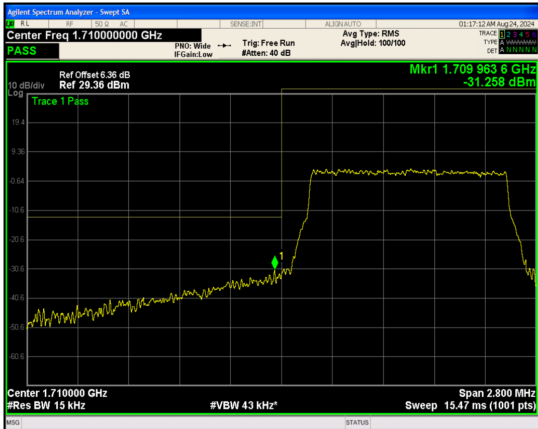
Band66 QPSK BW=1.4MHz Channel=132665 RB Size=6 Position=#0
