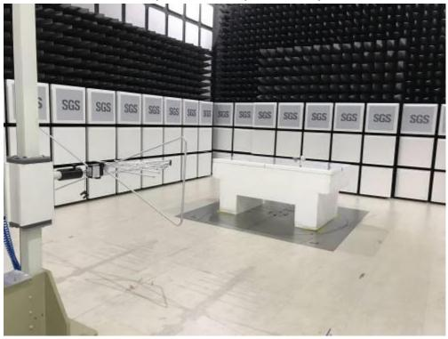
Radiated Emissions (Above 1GHz) Test Setup
