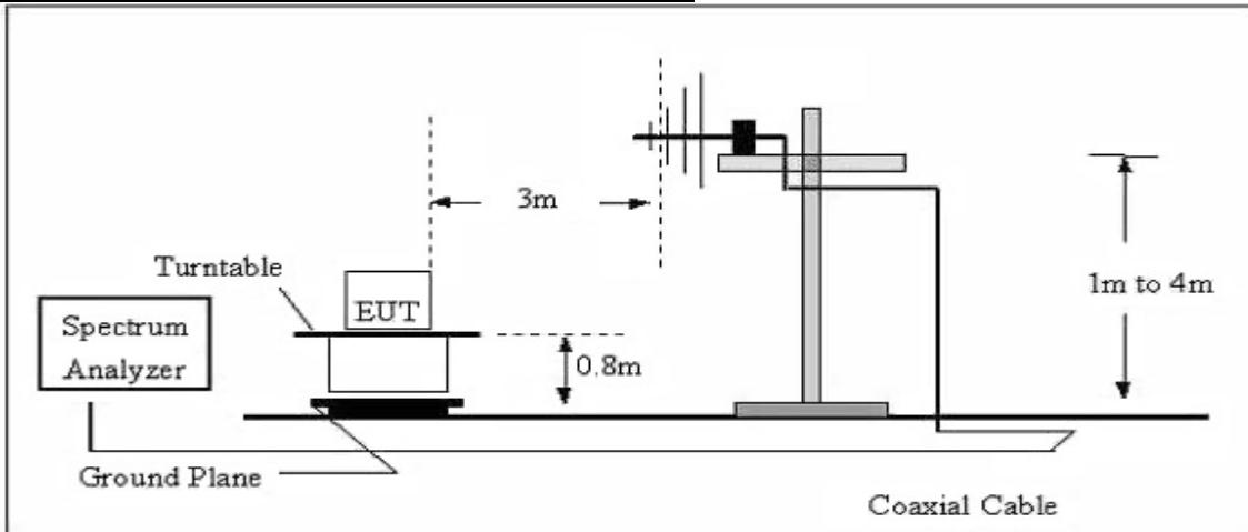
Radiated emission test-up frequency above 1GHz
