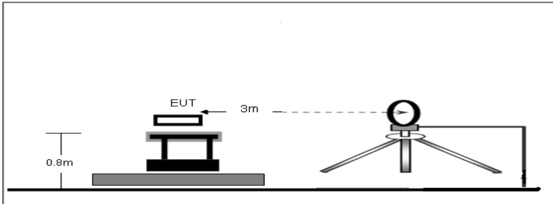
Radiated Emission Test-Up Frequency 30MHz~1GHz
