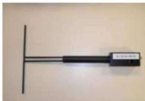
Figure 1 – Satimo COMOSAR Validation Dipole
