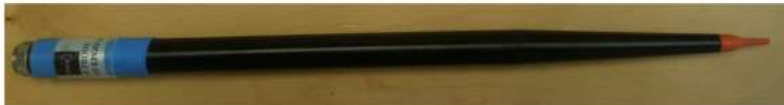
Figure 1 – MVG COMOSAR Dosimetric E field Dipole
