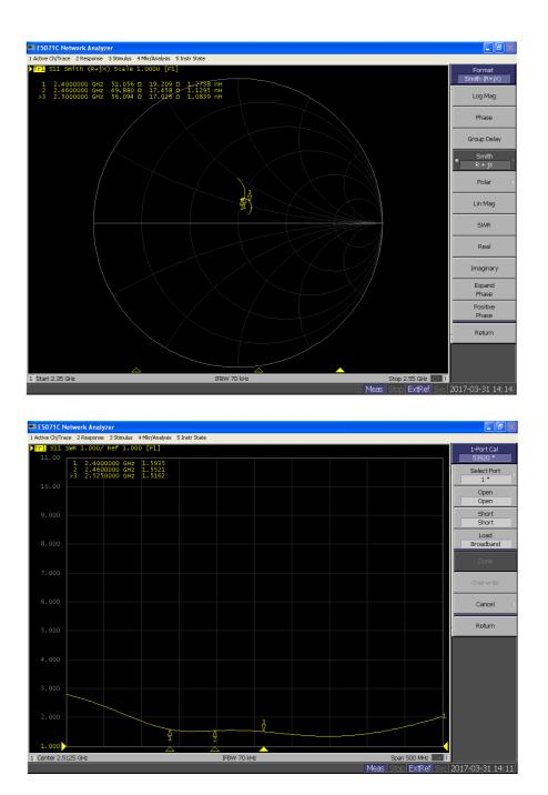
The antenna is sensitive to the size of the PCB RF ground layer and the plastic shell of the product. The antenna can be modeled as an LC resonator whose resonant frequency decreases when L(inductance) or C(capacitance) is increased. Larger radio frequency layers and plastic enclosures increase the effective capacitance, reducing the resonant frequency. Adjust the matching parameters according to the actual installation situation.
