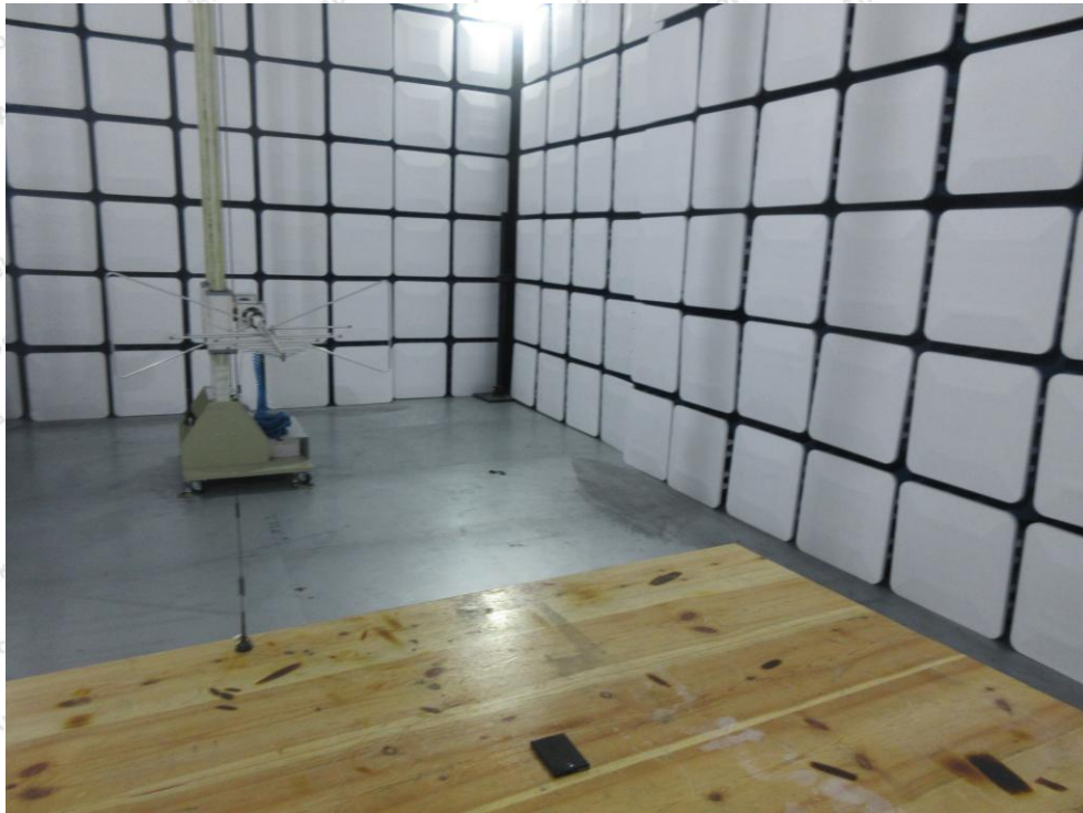
Photo of Radiation Emission Test
