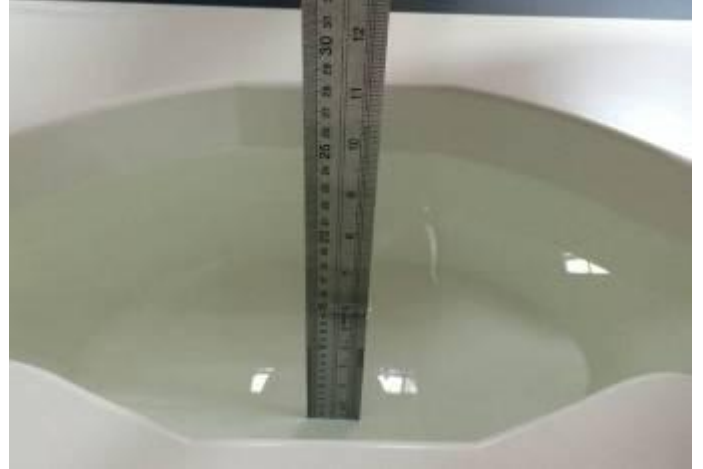
Body Position with 5000MHz liquid depth (15.2cm)
