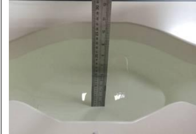
Body Position with 2450MHz liquid depth (15.4cm)
