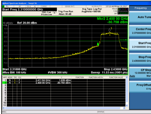
802.11n20: Band Edge-High Channel
