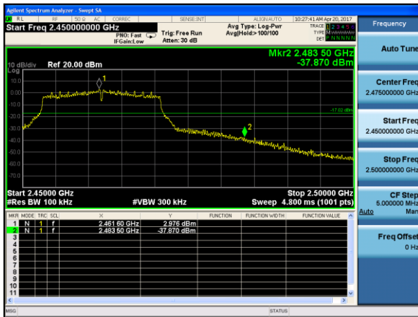
802.11n20: Band Edge-High Channel
