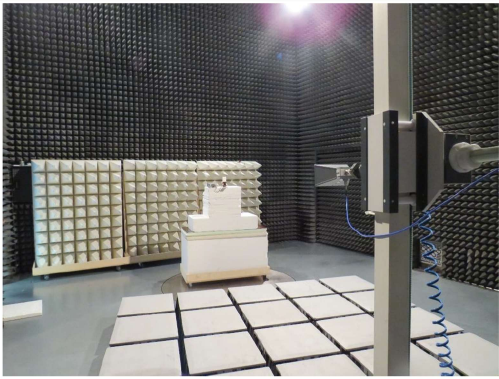
Test Setup Radiated Emissions 1 - 6.5 GHz
