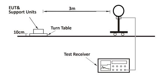
For Radiated emission 30MHz to 1GHz:
