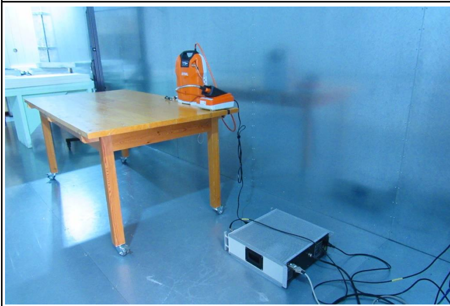
Test Set-up conducted emission
