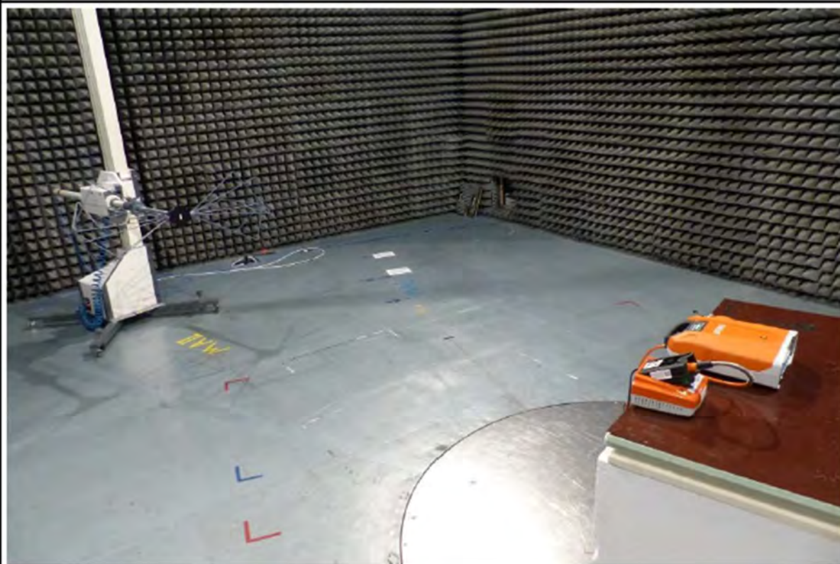
Test Setup EUT Configuration 2: 30-200MHz
