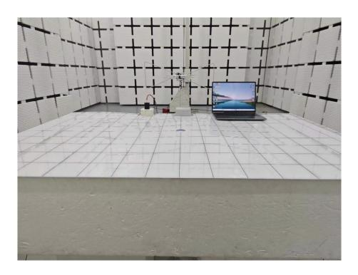
**Set-up for Radiated Spurious Emission, Above 1GHz**
