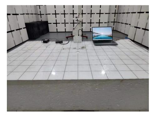
Set-up for Radiated Spurious Emission, Below 1GHz
