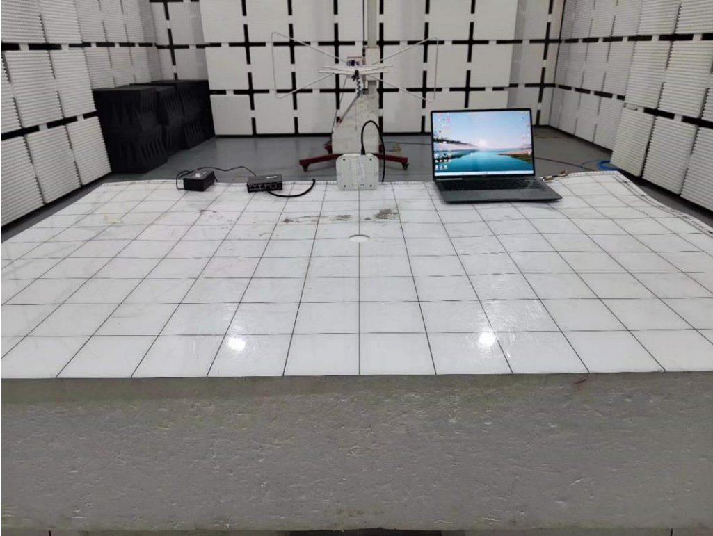
Set-up for Radiated Spurious Emission, Above 1GHz
