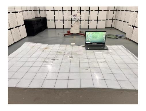
Set-up for Radiated Spurious Emission, Above 1GHz
